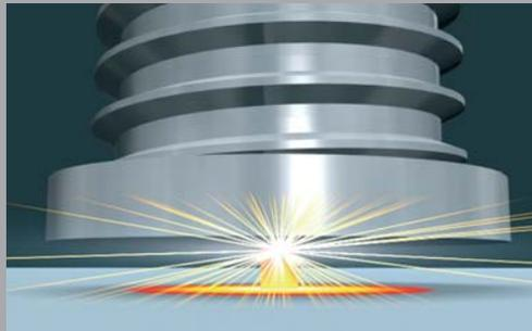
An arc is ignited between the face of stud and the surface of a work piece.
