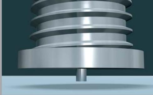
Joining of stud-type welding elements with a diameter M3 to M10 (dia. 2 to 10 mm) onto thin sheets, min. 0.5 mm. Mild steel, stainless, steel, aluminum and brass.
