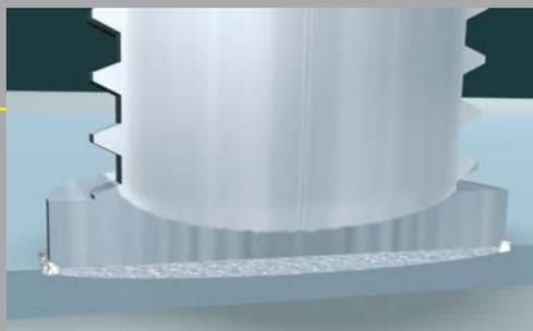
As a result, an even and complete joint is achieved with a strength which is above the strength of stud and base material. The low thermal load provides welding onto thin sheets without damage to the rear side.
