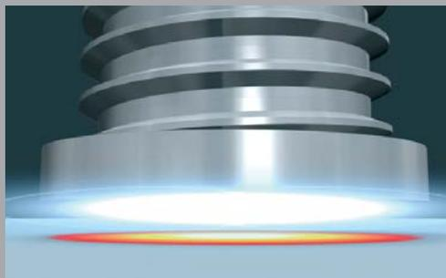
Both parts are melted, the stud is gently pressed against the work piece and then joined together.
